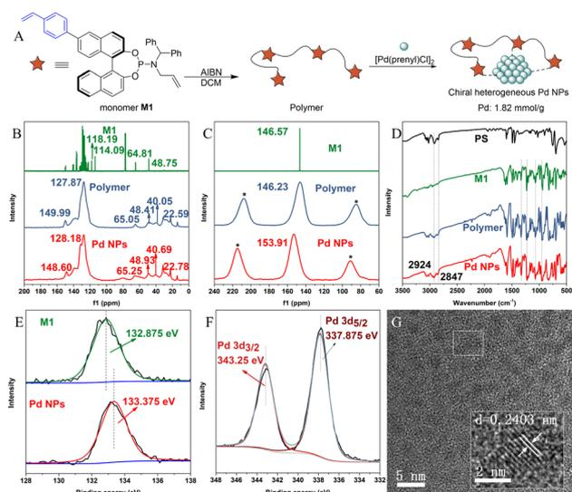
Fig. 2 Catalyst synthesis and characterization. (A) Synthesis of the chiral Pd NP catalyst; (B) solid state <sup>13</sup>C NMR spectra of **M1**, the polymer, and Pd NPs; (C) solid state <sup>31</sup>P NMR spectra of **M1**, the polymer, and Pd NPs; (D) FT-IR spectra of PS, **M1**, the polymer and Pd NPs; (E) P 2p of XPS analysis for **M1** and Pd NPs; (F) Rh 3d of XPS analysis for Pd NPs; (G) TEM of Pd NPs.
