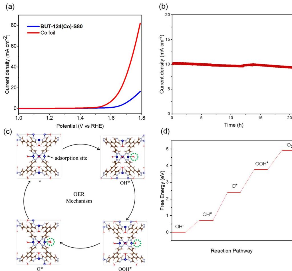
Fig. 4 (a) LSV curves of Co foil and BUT-124(Co)-S80 in a solution of 1 M KOH. (b) The chronopotentiometry curves of BUT-124(Co)-S80 at an overpotential of 393 mV in 1 M KOH solution. (c) Schematic illustration of the proposed OER mechanism. Color code: Co, blue; C, brown; N, gray; O, red; H, white. (d) The free energy profile for the OER pathway.
