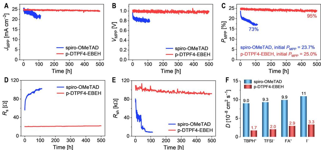
Fig. 7 (A–C) Photovoltaic parameters obtained from maximum power point (MPP) tracking under simulated AM1.5G irradiation at 100 mW cm<sup>-2</sup>: (A) photocurrent density ( $J_{MPP}$ ); (B) photovoltage ( $V_{MPP}$ ); (C) power conversion efficiency ( $P_{MPP}$ ). (D and E) Evolution of series resistance ( $R_s$ ) and shunt resistance ( $R_{sh}$ ) over time during MPP tracking. (F) Diffusivities of ions within the hole transport layer at 45 °C.
