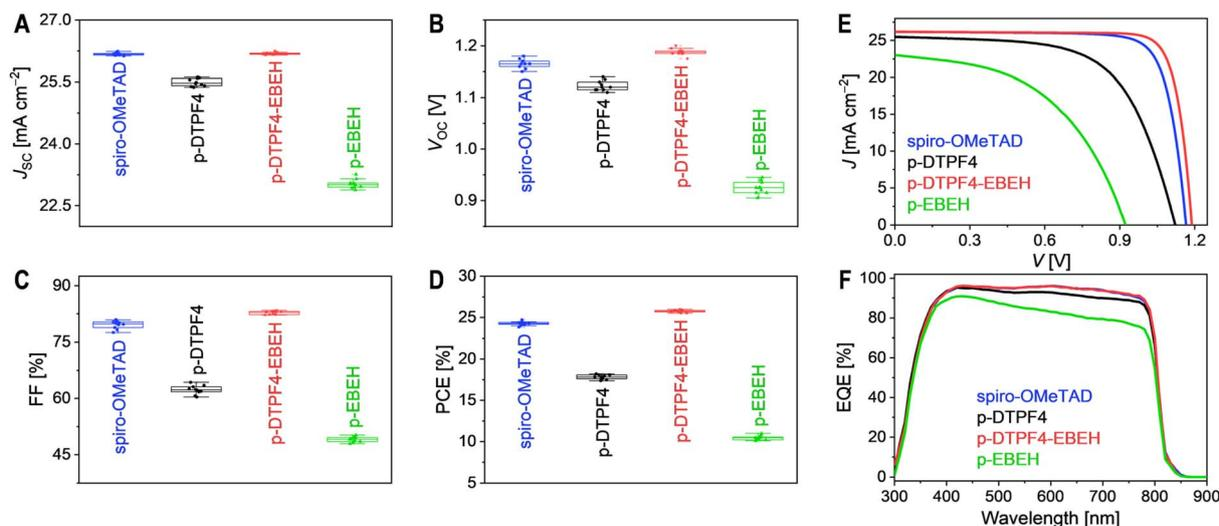
Fig. 3 (A–D) Statistical analysis of photovoltaic parameters of PSCs fabricated with varying hole transport layers under simulated AM1.5G irradiation at 100 mW cm<sup>-2</sup>: (A) short-circuit photocurrent density ( $J_{sc}$ ); (B) open-circuit voltage ( $V_{oc}$ ); (C) fill factor (FF); (D) power conversion efficiency (PCE). (E) Representative photocurrent density–voltage ( $J-V$ ) curves. (F) External quantum efficiency (EQE) spectra.
