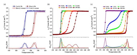
Fig. 4 Variation of the magnetic properties of framework 1 under  $CO_2$  adsorption under  $H_{dc} = 1$  kOe. (a) Magnetic susceptibility plots in the absence of any gas (open circles) and under 100 kPa He gas (filled circles). (b) The  $CO_2$  pressure dependence of the magnetic susceptibility measurements in cooling and (c) heating mode. First derivative plots are displayed at the bottom.
