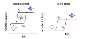
**Scheme 1** (Left) Breathing effect vs. (right) gating effect in gas adsorption of porous coordination polymers.
