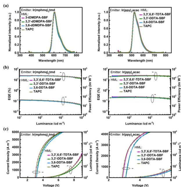
Fig. 3 OLED device performances. (a) Electroluminescence spectra at a luminance of 1000 cd m<sup>-2</sup>, (b) luminance and current density versus voltage curves, and (c) EQE and power efficiency versus luminance curves of red (left) and green (right) PhOLED devices.
