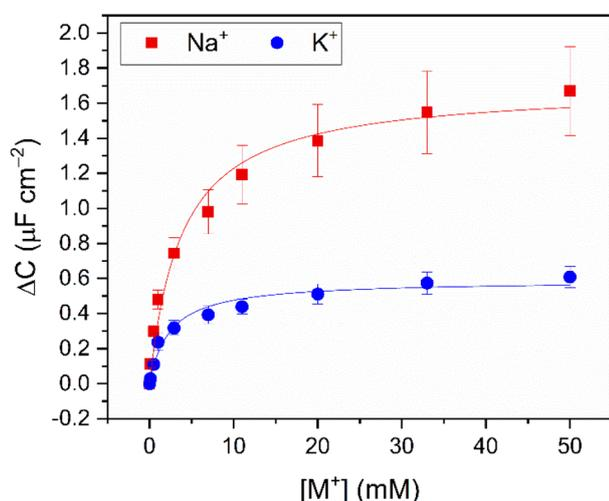
Fig. 2 Response isotherms of **B15C5**<sub>SAM</sub> determined from the shift in  $C'$  in response to increasing concentrations of  $\text{Na}^+$  (red squares) and  $\text{K}^+$  (blue circles) in H<sub>2</sub>O with 100 mM TEACl as supporting electrolyte, under static conditions. Isotherms were fitted to a Langmuir model (see ESI Section S1.6 for further details, and eqn (S1)†). Errors represent one standard deviation of three independent repeats.
