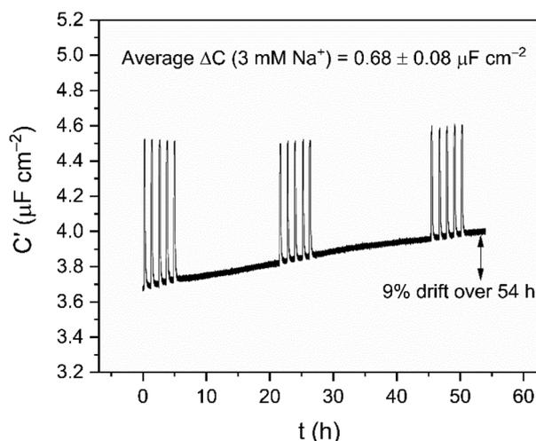
**Fig. 5** Long term cation sensing experiment conducted over 54 h in water (100 mM TEACl as supporting electrolyte). Responses of **B15C5<sub>SAM</sub>** to 3 mM Na<sup>+</sup> are shown as spikes in the sensogram.
