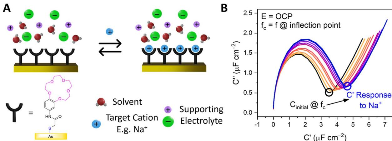
Fig. 1 (A) Schematic depiction of **B15C5**<sub>SAM</sub> in the absence (left) and presence (right) of a specific target. (B) Capacitive Nyquist plots of **B15C5**<sub>SAM</sub> in H<sub>2</sub>O, 100 mM TEACl conducted at fixed OCP. Changes in  $C$  are measured at the inflection point of each Nyquist plot (corresponding to frequency,  $f_c$ ) upon addition of increasing concentrations of NaCl up to 50 mM (blue) in static solution.
