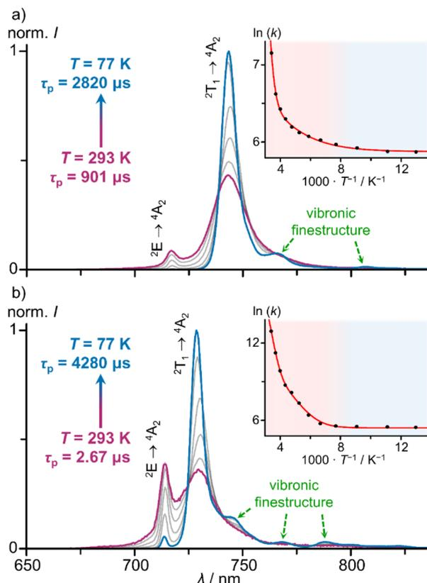
Fig. 4 Integration area normalised low temperature emission spectra ( $\lambda_{\text{exc}} = 450$  nm) of (a)  $[1^O]^{3+}$  and (b)  $[1^S]^{3+}$  in a mixture of ethanol/methanol (3 : 2 v/v) between 77 and 293 K under deaerated conditions. Insets show corresponding Arrhenius plots of the photoluminescence rate constants  $k(T)$  with fit and coloured backgrounds for temperature ranges of liquid (red) and frozen solvent mixture (blue).
