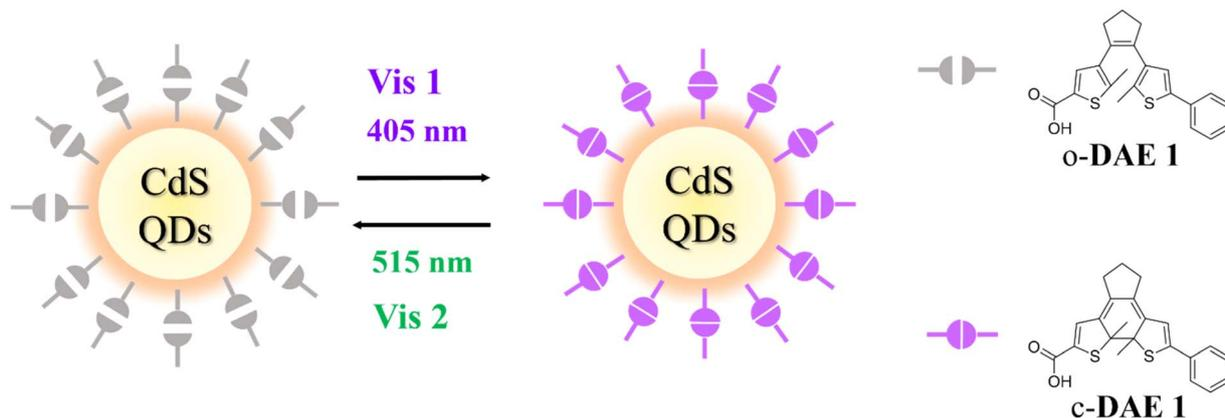
Scheme 1 Schematic illustration of all-visible light activated modulation of the CdS QDs and carboxylated DAE 1 in the open and closed forms.
