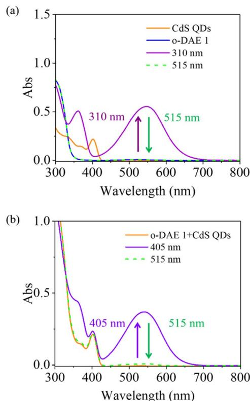
Fig. 1 Absorption spectra of CdS QDs and DAE 1 responding to light irradiation. (a) Absorption spectra of individual CdS QDs (0.5  $\mu\text{M}$ ) and DAE 1 (50  $\mu\text{M}$ ) in toluene. (b) Absorption spectra of the mixture of CdS QDs (0.5  $\mu\text{M}$ ) and DAE 1 (50  $\mu\text{M}$ ) in toluene. DAE 1 was irradiated with 310 nm, 405 nm and 515 nm light to the respective photostationary states.
