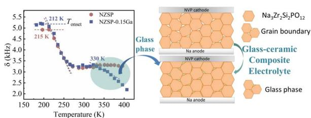
The glass phase in the grain boundary of  $\text{Na}_3\text{Zr}_2\text{Si}_2\text{PO}_{12}$ , created by gallium modulation
