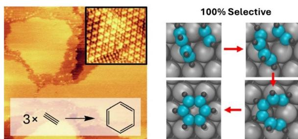
**100% selective cyclotrimerization of acetylene to benzene on Ag(111)**
