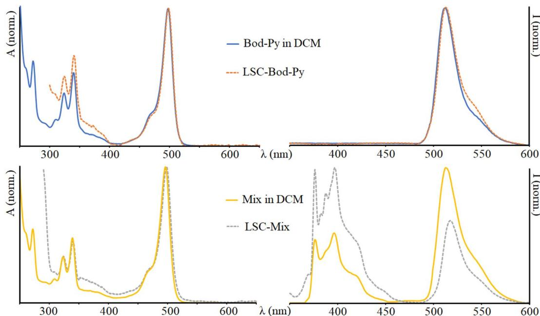
Fig. 2 Absorption (on the left) and emission (on the right) spectra of **Bod-Py** and **Mix** in DCM and in the LSC.  $\lambda_{exc} = 350$  nm. The spectra of the other species are illustrated in the ESI<sup>†</sup>.
