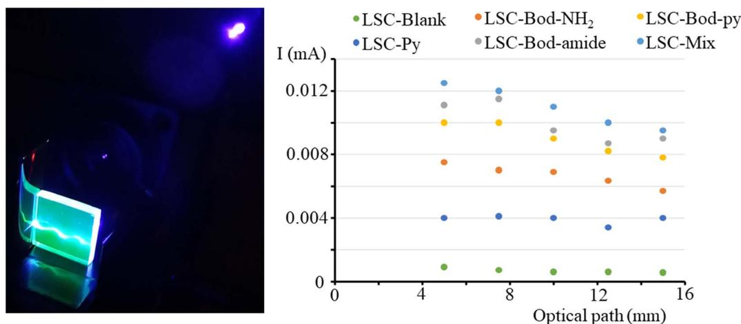
Fig. 6 In the left panel: photograph of the experimental set-up used for monitoring the photocurrent vs. optical path; a 406 nm laser is irradiating **LSC-Bod-Py** and the emission light waveguide inside the LSC matrix is visible. In the right panel: diagram illustrating the influence of the optical path on the photocurrent of the LSC-PV device.
