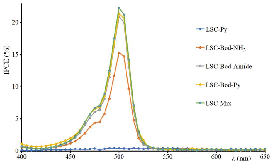
Fig. 7 IPCE spectra of the fabricated LSC.
