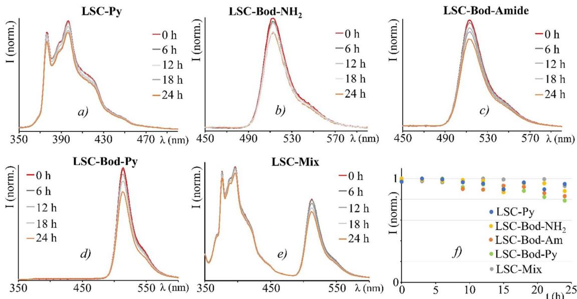
Fig. 5 Panels (a), (b), (c), (d) and (e) show emission spectra ( $\lambda_{\text{exc}} = 330$  nm) of the studied chromophores in the LSC after 24 h of irradiation with a AM 1.5G solar simulator. In panel (f): normalized trend of the luminescence intensities of the corresponding emission band maximum.
