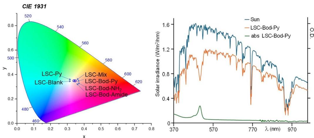
**Fig. 4** In the left panel: position of the fabricated LSCs in the CIE 1931 chromaticity diagram. In the right panel: in blue, the solar spectrum using an AM 1.5G filter; the orange line represents the transmission spectrum of the solar simulator filtered by LSC-Bod-Py; the absorption spectrum of LSC-Bod-Py is shown in green. LSC-Bod-Py is selected here as a representative example. The spectra of the other prepared LSCs are illustrated in Fig. S6 in the ESI.†
