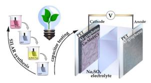
Flexible laser-induced graphene-based electrodes modified with cobalt-manganese hexacyanoferrate as cathode materials for asymmetric supercapacitors
