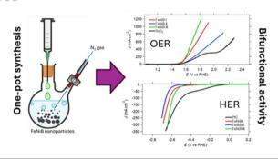
Scalable one-pot synthesis of amorphous ironnickel-boride bifunctional electrocatalysts for enhanced alkaline water electrolysis
