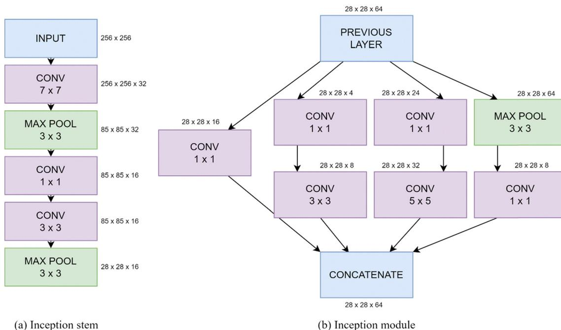
Fig. 2 Schematics of an example (a) inception stem and (b) module showing the kernel sizes of each convolutional and pooling layer.
