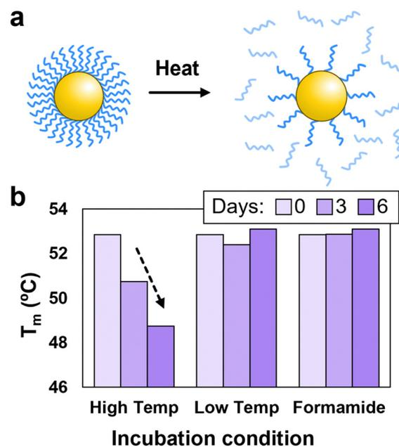
Fig. 4 PAE viability in different environments. (a) Schematic of DNA anchors desorbing from gold cores during heating. (b)  $T_m$  is plotted for PAEs incubated in different conditions over the course of 6 days. While PAEs held at elevated temperatures (60 °C) display a significant drop in  $T_m$  in this time, those held at room temperature with or without formamide remain constant.
