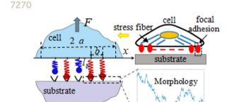
A viscoelastic-stochastic model of cell adhesion considering matrix morphology and medium viscoelasticity
