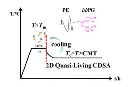
Two-dimensional (2D) quasi-living crystallizationdriven self-assembly of polyethylene-bhyperbranched polyglycidol diblock copolymers in solution
