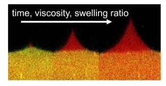
Phase separation dynamics in wetting ridges of polymer surfaces swollen with oils of different viscosities
