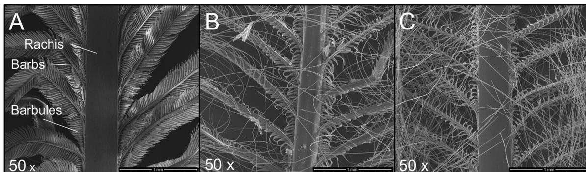
Fig. 7 SEM of chicken feathers treated with trypsin. (A) Control without trypsin, (B) trypsin hydrolysis for 16 h, (C) trypsin hydrolysis for 48 h. The magnification is 50 $\times$ .
