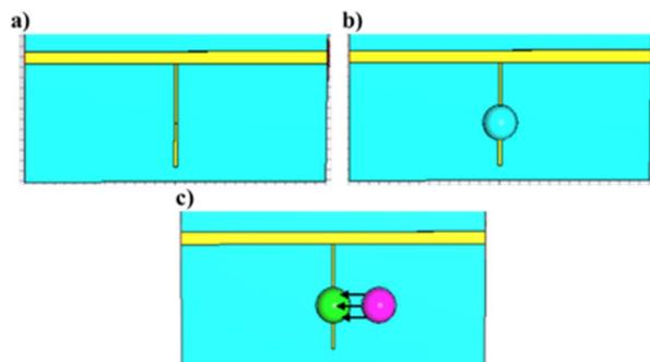
Fig. 8 Numerical simulation setup (CST software) of the ChCl/U dielectric characteristics ( $\epsilon_r$  and  $\text{tg}\delta$ ) based on the quarter-wavelength stub resonator measurements with (a) an unfilled gap, (b) a gap filled with a water droplet (see the blue half-sphere) and (c) DES droplet deposition (see the green half-sphere) exposed to HCl vapor (see the pink half-sphere).
