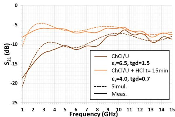
Fig. 11 Comparison of the simulated and measured transmission coefficient magnitudes of the 50  $\Omega$  transmission line with its gap filled with a ChCl/U DES droplet considered as a sensitive layer, before and after 15 min exposure to HCl vapor.
