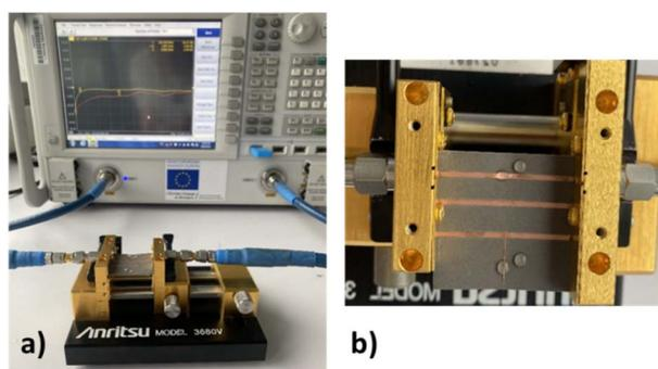
Fig. 4 (a) Experimental setup (VNA + V cell) used to validate the DES-based microwave gas sensor concept and to retrieve the dielectric characteristics ( $\epsilon_r$  and  $\text{tg}\delta$ ) of the DES sensitive material; (b) details of the V-Anritsu cell after the deposition of the DES and HCl droplets.
