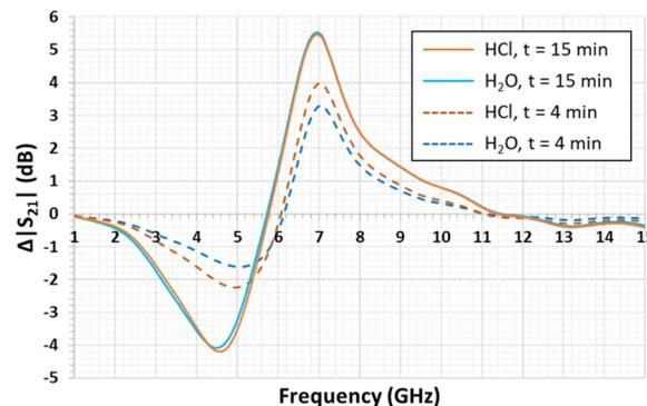
Fig. 7 Magnitude differences of transmission coefficients ( $\Delta S_{21}$ ) versus frequency values for exposure to HCl (orange lines) or water (blue lines) at two exposure times of 4 min (dashed lines) and 15 min (straight lines). The ChCl/U DES is used as a sensitive material.
