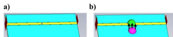
Fig. 10 Numerical simulation setup (CST software) of the 50  $\Omega$  transmission line with (a) an unfilled gap and (b) a gap filled with the ChCl/U DES droplet (see the green half-sphere) and exposed to HCl vapors (see pink half-sphere).
