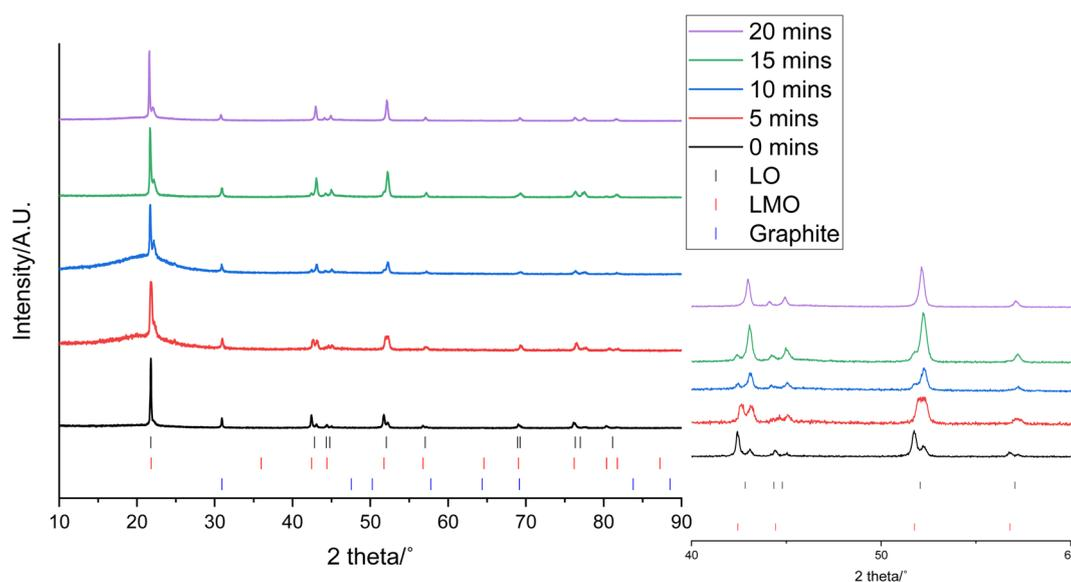
Fig. 3 XRD patterns of 0.3 g end-of-life cathode after leaching in 10 mL of 1 M citric acid for 0 (black), 5 (red), 10 (blue), 15 (green) and 20 minutes (purple) (Co K $\alpha$ ). Tick marks correspond to LO (black), LMO (red) and graphite (blue).
