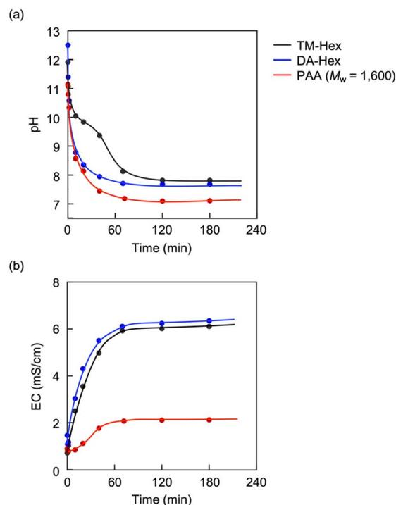
Fig. 7 Variations in (a) pH and (b) EC upon introducing  $\text{CO}_2$  into solutions of TM-Hex,<sup>54</sup> DA-Hex and PAA.  $[\text{NR}_2]_0 = 2.63 \text{ mol L}^{-1}$  for the pH measurement and  $0.117 \text{ mol L}^{-1}$  for the EC.  $\text{R} = \text{CH}_3$  for TM-Hex and H for DA-Hex and PAA.  $\text{CO}_2$  flow rate =  $250 \text{ mL min}^{-1}$ .
