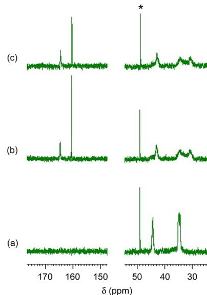
Fig. 3  $^{13}\text{C}$  NMR spectra. (a) PAA with  $M_w = 15\,000$ , (b) the CA-captured PAA in solution after  $\text{CO}_2$  introduction for 1 h and (c) the CA-captured PAA isolated. Solvent:  $\text{D}_2\text{O}$ . \* $\text{CH}_3\text{OH}$  standard.
