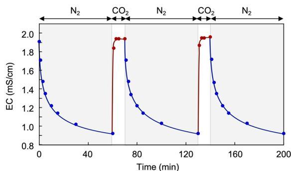
Fig. 14 Repetitive changes in EC and pH of the CA-captured PAA by alternating  $CO_2/N_2$  introductions.  $[AA]_0 = 0.116 \text{ mol L}^{-1}$ ,  $M_w = 15\ 000$ .
