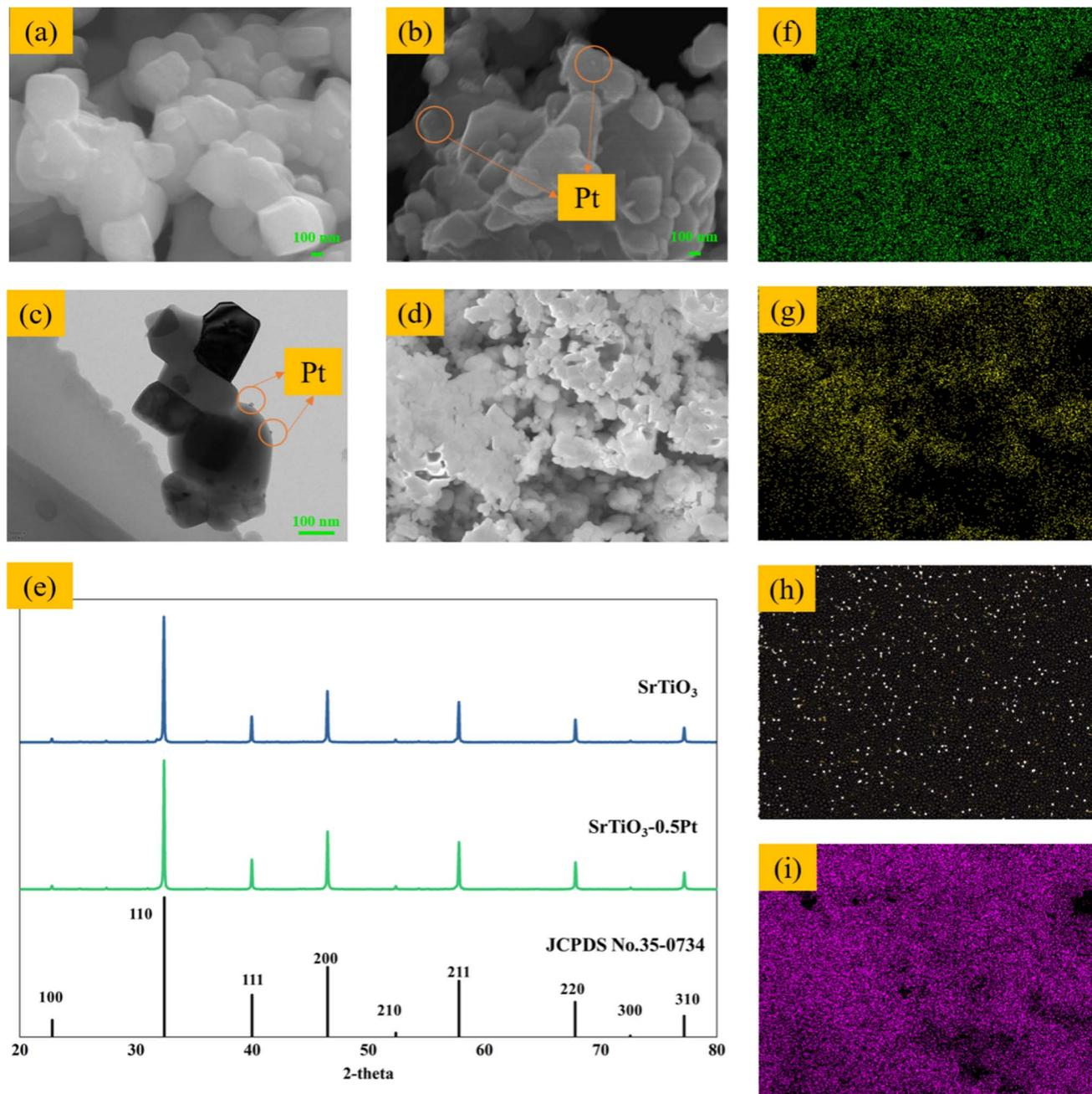
Fig. 2 Characterization of  $\text{SrTiO}_3\text{-Pt}$ . (a) SEM image of  $\text{SrTiO}_3$ , (b) SEM image of  $\text{SrTiO}_3\text{-0.5Pt}$ , (c) TEM image of  $\text{SrTiO}_3\text{-0.5Pt}$ , (d) area scanned by EDS, (e) XRD patterns for the  $\text{SrTiO}_3$  and  $\text{SrTiO}_3\text{-Pt}$  catalysts, (f) EDS image of elemental Ti, (g) EDS image of elemental O, (h) EDS image of elemental Pt, and (i) EDS image of elemental Sr.
