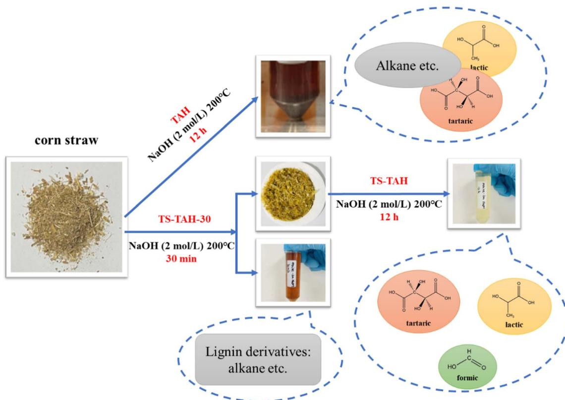
Fig. 1 Two-stage thermo-alkaline hydrolysis (TS-TAH) of corn straw.
