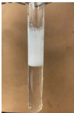
Fig. 2 Foam test for soapnut extract solution.
