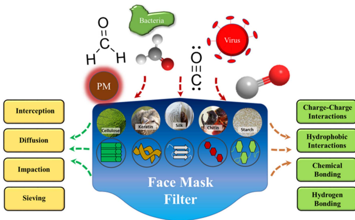
Fig. 13 Materials for biopolymer-based filtration made from various protein and polysaccharide sources. Particulate matter (PM), viruses, bacteria, and smoke pollutants can all be filtered out due to their particular surface chemistries and varied molecular interactions. 150 Reprinted with permission from ACS Publication (2021).
