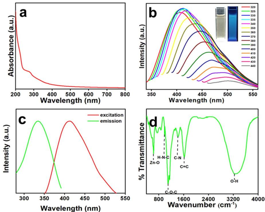
Fig. 1 (a) UV-Vis spectrum of Zn-Cdots dispersed in water at a concentration of  $0.25 \text{ mg mL}^{-1}$ . (b) Excitation-dependent emission of Zn-Cdots dispersed in water at  $0.5 \text{ mg mL}^{-1}$  concentration (inset: images of aqueous solution of Zn-Cdots under daylight and UV light). (c) Excitation (wavelength  $330 \text{ nm}$ ) spectrum of Zn-Cdots corresponding to the  $411 \text{ nm}$  emission peak. (d) FTIR spectrum of Zn-Cdots.
