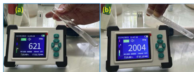
Fig. 4 (a) Test tube containing aqueous solution of the soda ash synthesized. (b) Test tube containing acidified solution of the soda ash.
