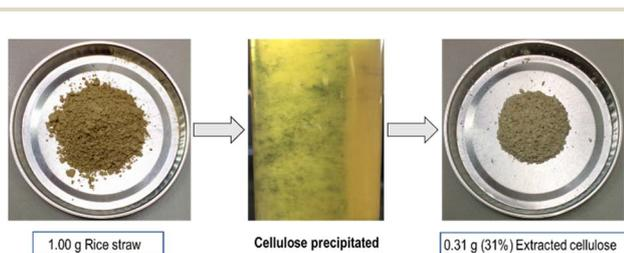
Fig. 2 Isolation of raw cellulose from rice straw.
