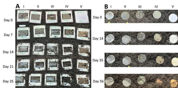
**Fig. 8** Biodegradability test of (A) inside the soil (films are fixed in a Dia frame), and (B) on the soil surface. (I) PE foil, (II) PLA foil, (III) Cellophane "Natureflex", (IV) RC film 1, (V) paper.
