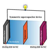
An improved Hummers method derived graphene oxide wrapped ZIF-8 polyhedron derived porous heterostructure for symmetric supercapacitor performance
