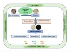
Incorporating biochar to make hydrogel composites with improved structural properties, valorized from waste-paper mill sludge and forestry residues using energy efficient protocols
