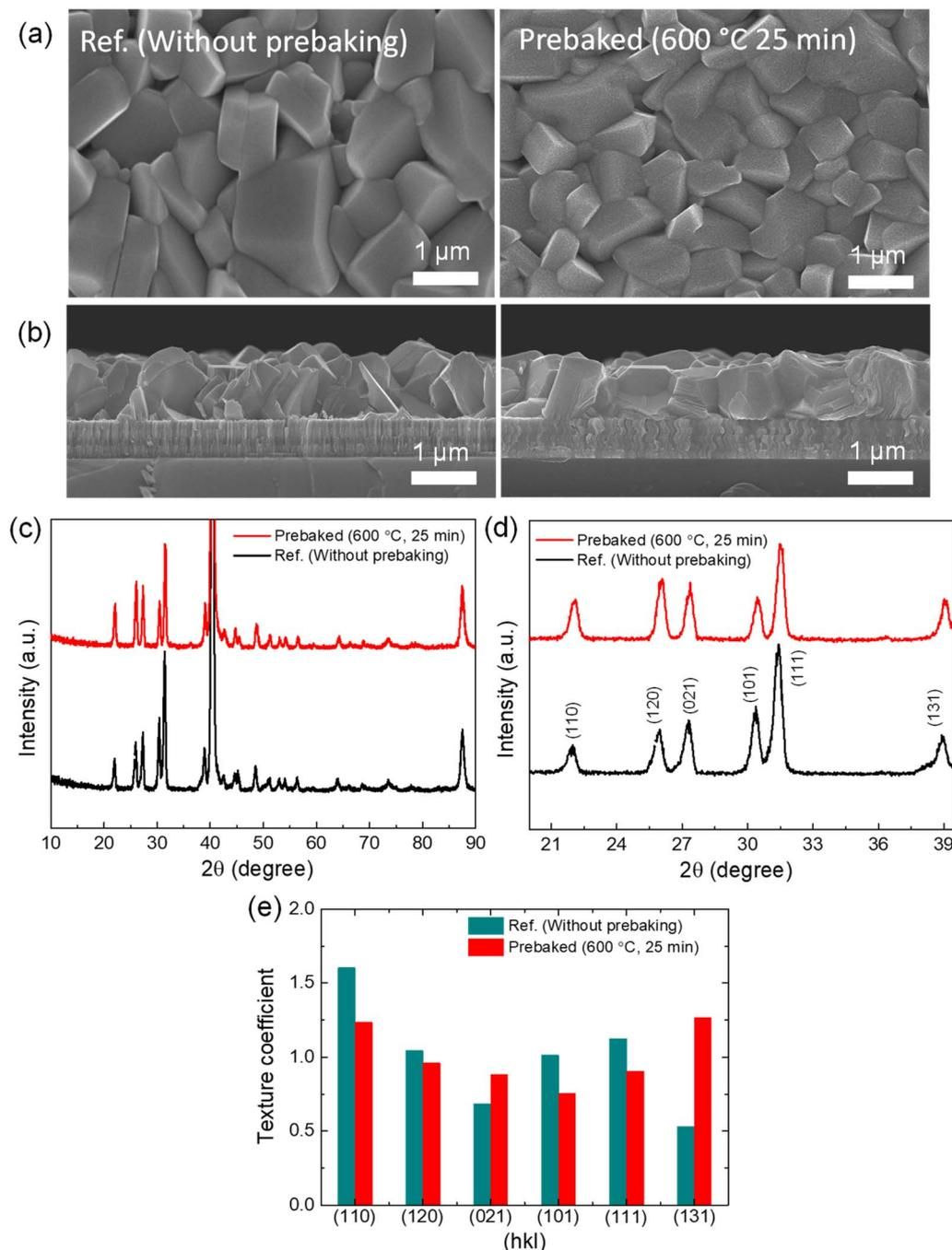
Fig. 2 SEM image of the without prebaking (W.B.; ref.) and 600 °C-prebaked SnS: (a) top surface morphology, (b) cross-section, (c) X-ray diffraction (XRD) pattern of the W.B. and prebaked source films in the  $2\theta$  range of 10 to 90°, (d) XRD pattern of the W.B. and prebaked source films in the  $2\theta$  range of 20 to 40°, and (e) the calculated texture coefficient of different planes.
