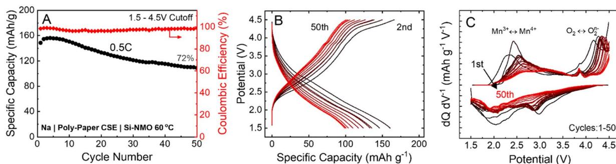
Fig. 4 (A and B) Cycling stability and voltage profiles of Si-NMO solid-state cells at C/2 rate (80  $\mu\text{A cm}^{-2}$ ), exhibiting 72% capacity retention after 50 cycles. (C) Differential capacity curves ( $dQ/dV$ ) of the cells with a clear Mn<sup>3+</sup> to Mn<sup>4+</sup> transition at  $\sim 2.80$  V.
