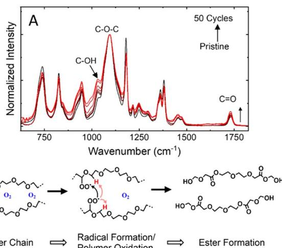
Fig. 6 (A) FTIR spectra of the pristine poly-paper CSE and *ex situ* measurements to identify the effects of cycling on the CSE. (B) Schematic of the mechanism of ether oxidation that occurs in the cell during cycling. Sodium ions have been removed from the figure to improve the clarity of the oxidation mechanism.
