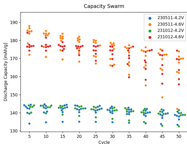
Fig. 9 A comparison of the capacity degradation of selected cells in the two cell batches assembled using Aurora, with one batch (231012) tested in-band using AiiDALab-Aurora, and the second batch (230511) tested out-of-band of AiiDA, using EC-Lab. Only two of the four sub-batches of cells shown, a plot of all retrieved data is available in the ESI, see Fig. S6.†
