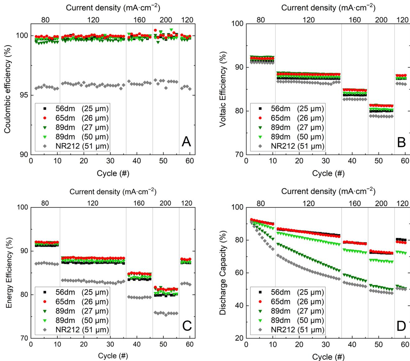
Fig. 7 Cycling performance of Nafion™ NR212 and the HMT-PMBI membranes with coulombic efficiency (A), voltaic efficiency (B), energy efficiency (C) and the normalized discharge capacity (D).
