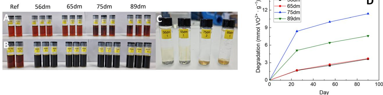
Fig. 5 Chemical stability analysis of HMT-PMBI in the 1.6 M VO<sub>2</sub><sup>+</sup> electrolyte with the immersed samples at the start of the test (A), at the end of the test after 90 days (B), post-test immersed in 3 M NaCl (C) as well as the degradation of the HMT-PMBI derivatives described in mmol VO<sub>2</sub><sup>+</sup> formed per gram of polymer over these 90 days (D).
