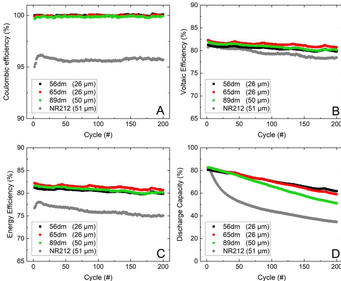
Fig. 8 The cycling performance of the HMT-PMBI variants and Nafion™ NR212 over 200 cycles at  $200 \text{ mA cm}^{-2}$ , with the coulombic efficiency (A), voltaic efficiency (B), energy efficiency (C) and normalized discharge capacity (D).
