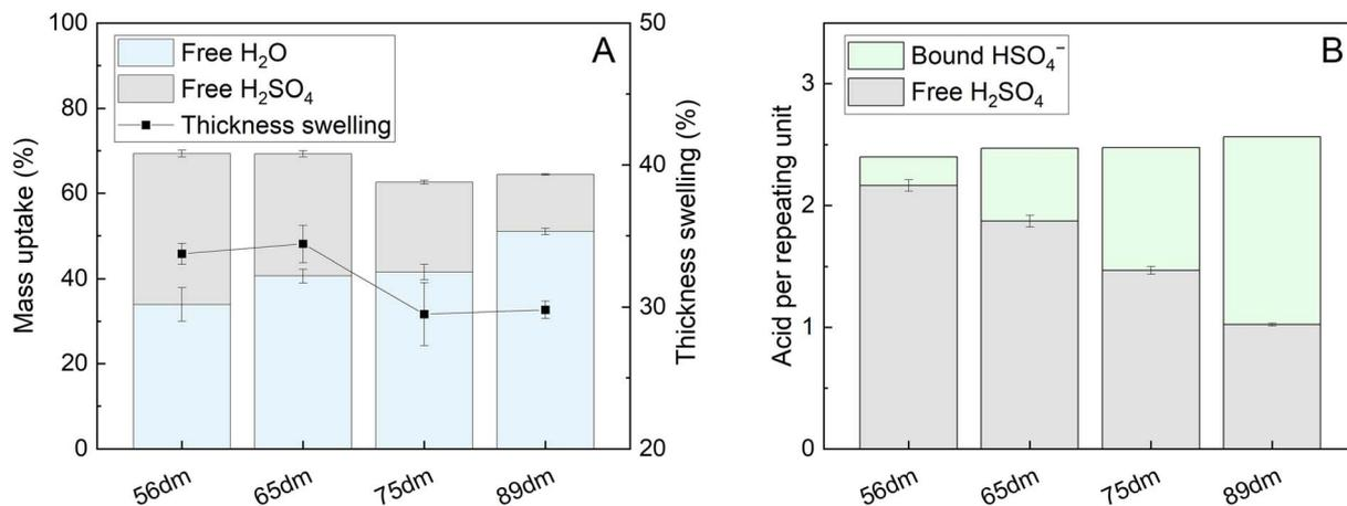
Fig. 3 Water uptake, acid uptake and thickness swelling of HMT-PMBI membranes with various degrees of methylation (dm) upon immersion in 2 M H<sub>2</sub>SO<sub>4</sub> (A) and the corresponding acid content per repeating unit (B).
