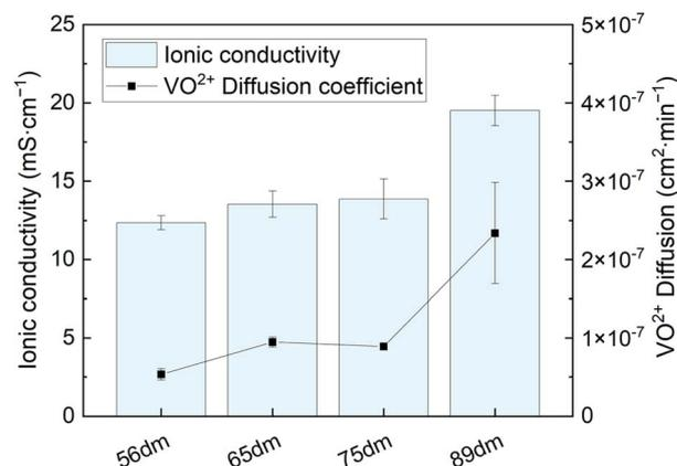
Fig. 4 Through-plane ionic conductivity in a 1.6 M vanadium electrolyte (SoC -50%) and VO<sup>2+</sup> diffusion coefficient of the different HMT-PMBI variants.
