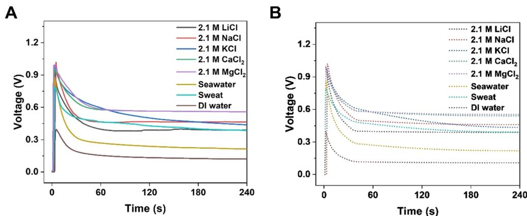
Fig. 5 Numerical simulation of the electrical performance of KB6/W-based HENGs with various salts of 2.1 M. Experimental (A) and simulated (B) real-time open-circuit voltages ( $V_{OC}$ ); A is reprinted with permission from,<sup>3</sup> copyright 2023, Elsevier.
