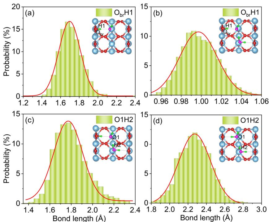
Fig. 3 Probability distributions of  $O_{br}H$  bond lengths in (a) a single water molecule and (b) monolayer systems, and IHB lengths (c) after and (d) before water dissociation in the monolayer system.
