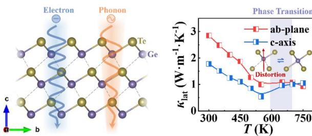
**Anisotropic thermoelectric properties of GeTe single crystals**
