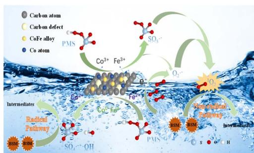
**Magnetic CoFe alloy–Co supported on mesoporous carbon as an efficient catalyst for the degradation of bisulfuron-methyl: insight into the effect of calcination temperature on carbon defects and singlet oxygen**
