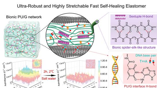
**Ultra-robust, highly stretchable and ambient temperature rapid self-healing polyurethane/graphene elastomers enabled by multi-type hydrogen bonds**
