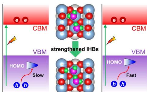
**Enhancement of hole capture and water dissociation on rutile TiO<sub>2</sub>(110) by intermolecular hydrogen bonding: time-domain *ab initio* study**
