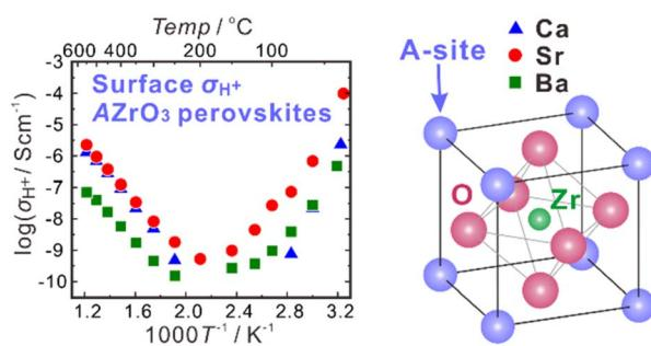
**Surface protonic conduction in porous alkaline earth zirconate perovskites  $\text{CaZrO}_3$ ,  $\text{SrZrO}_3$ , and  $\text{BaZrO}_3$**
