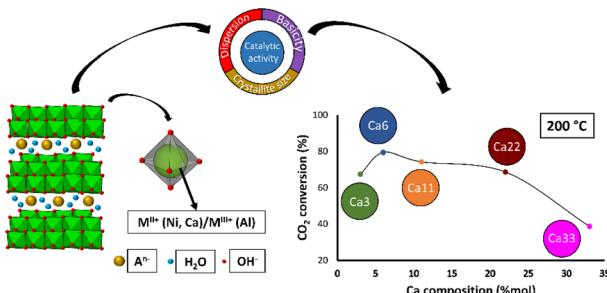
**Tuning the Ca content of Ni–Ca–Al layered-double hydroxide catalysts for low-temperature CO<sub>2</sub> methanation**
