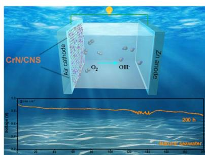
**Carbon nanosheet-supported CrN nanoparticles as efficient and robust oxygen reduction electrocatalysts in acidic media and seawater Zn-air batteries**
