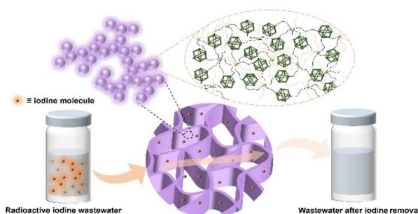
**Robust hydrogels with hierarchical porosities from the controlled assembly of metal-organic polyhedra for rapid removal of low-concentration aqueous iodine**
