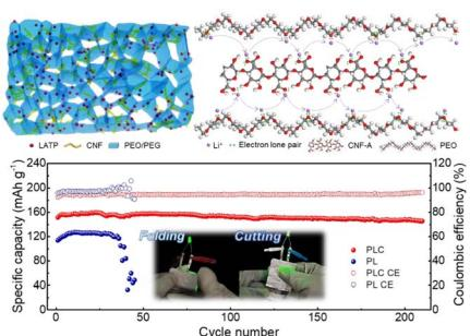
**High ionic conductivity of a flexible solid-state composite electrolyte for a lithium-ion battery**
