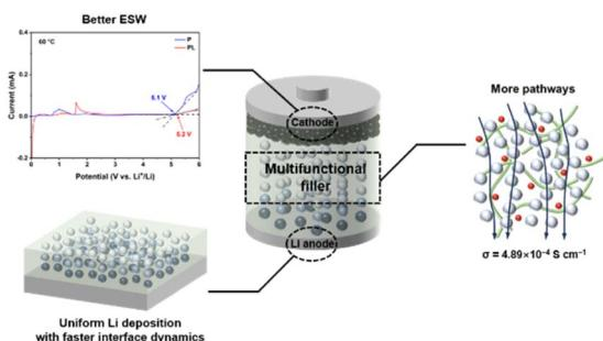
**Utilizing Li<sub>4</sub>Ti<sub>5</sub>O<sub>12</sub> as multifunctional filler in composite solid electrolyte for all-solid-state lithium metal battery**
