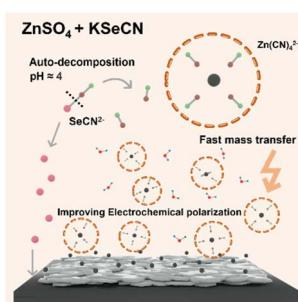
**Mediation of the electrochemical polarization for durable zinc anode**
