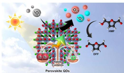
**Photocatalytic conversion of 5-hydroxymethylfurfural using mixed halide perovskite MAPbBr<sub>x</sub>Cl<sub>3-x</sub> quantum dots**
