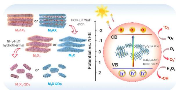
**Outstanding ROS generation ability and the mechanism of MXene quantum dots**
