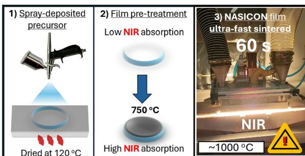
**A new approach for obtaining ceramic NASICON ( $\text{Na}_3\text{Zr}_2\text{Si}_2\text{PO}_{12}$ ) films sintered *in situ* by a sol–gel method, using spray deposition and near-infra red sintering**
