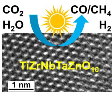
**Hybrid d<sup>0</sup> and d<sup>10</sup> electronic configurations promote photocatalytic activity of high-entropy oxides for  $\text{CO}_2$  conversion and water splitting**
