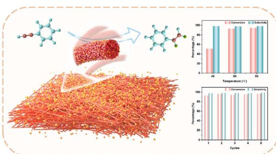
**Electron-deficient Pd nanoparticles on nitrogen-doped carbon nanofibers for high selectivity alkyne transfer semi-hydrogenation**
