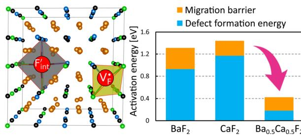
**Point-defect chemistry for ionic conduction in solid electrolytes with isovalent cation mixing**
