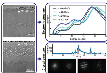
**Insights into defect kinetics, mass transport, and electronic structure from spectrum effects in ion-irradiated Bi<sub>2</sub>O<sub>3</sub>**
