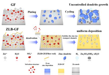
**Zein improved GF separator for dendrite-free aqueous zinc-ion batteries**
