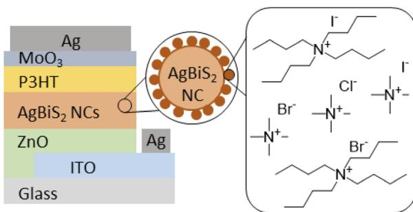
**Effect of different halide-based ligands on the passivation and charge carrier dynamics in AgBiS<sub>2</sub> nanocrystal solar cells**
