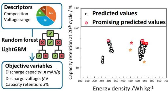
**Na[Mn<sub>0.36</sub>Ni<sub>0.44</sub>Ti<sub>0.15</sub>Fe<sub>0.05</sub>]O<sub>2</sub> predicted via machine learning for high energy Na-ion batteries**
