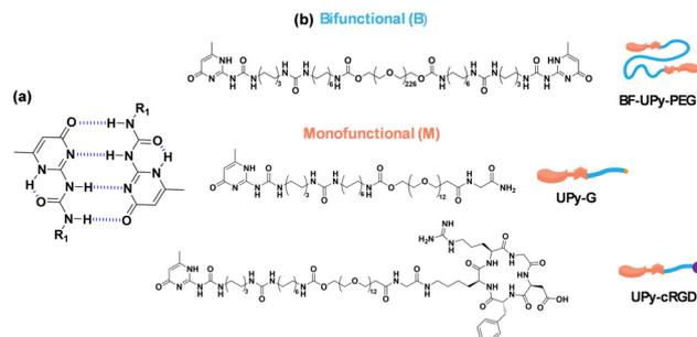
**Fig. 1** (a) Diagram showing the self-complementary quadruple hydrogen bonding between two UPy-units, where “R” represents the respective polymer linker. (b) Structures of bifunctional (B)-type and monofunctional (M)-type molecules as the supramolecular building blocks and additives.
