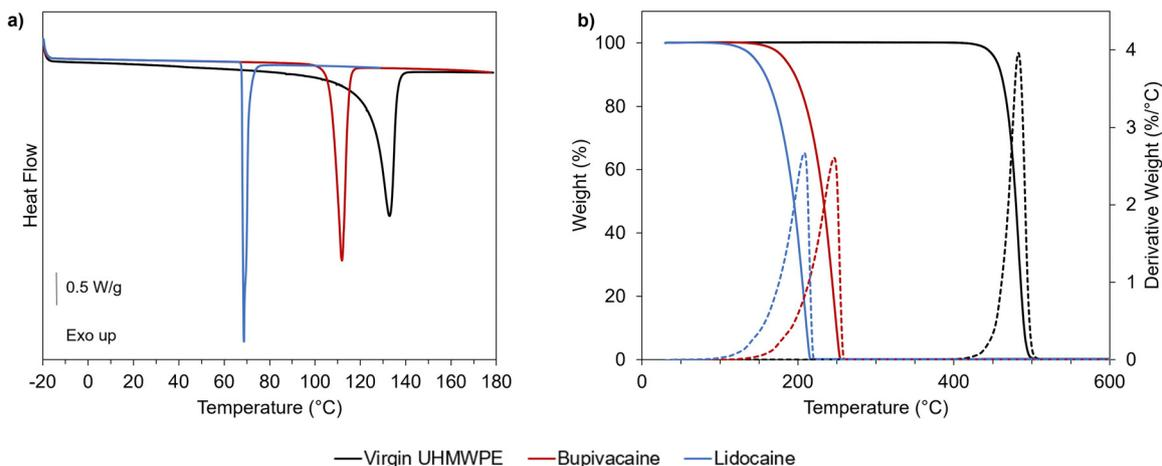
Fig. 3 Thermal and thermogravimetric behavior of UHMWPE and selected analgesic drugs. (a) DSC first heating scan and (b) TGA heating ramp ( $10\text{ }^{\circ}\text{C min}^{-1}$ ) for virgin UHMWPE (black line), bupivacaine (red line) and lidocaine (blue line). Dashed lines in (b) refer to the derivative weight curves.
