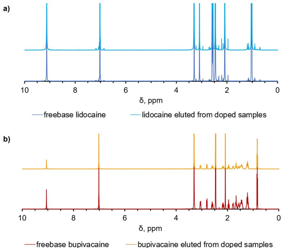
Fig. 5 Chemical stability of analgesics incorporated into UHMWPE by diffusion doping. Comparison between the  $^1\text{H}$  NMR spectra of the freebase stock solution and the drug eluted from the doped UHMWPE samples for (a) lidocaine and (b) bupivacaine.
