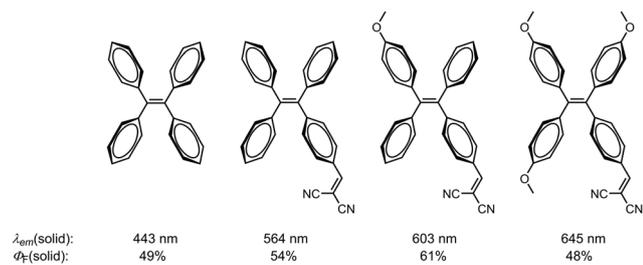
Fig. 1 Tunable luminescence of TPE-based AIEgens in the solid state.<sup>22</sup>
