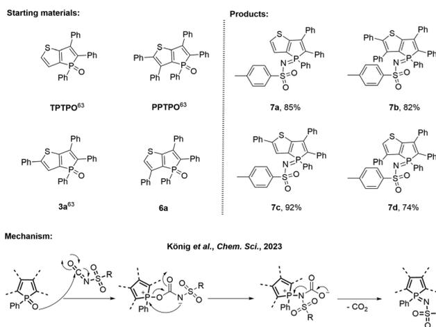
**Scheme 2** Transformation into the tosylimino phospholes **7a–d**, their isolated yields and the proposed mechanism.<sup>64</sup>
