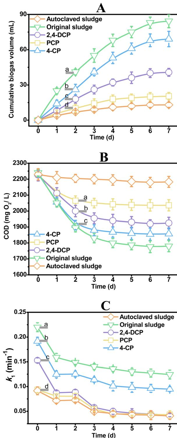
Fig. 5 The cumulative biogas (A) and chemical oxygen demand removal (B) during 7 days anaerobic digestion with 4-CP, DCP and PCP spiked, and (C) kinetics (presented as  $k_1$  of  $\Delta$ Hue due to resazurin reduction by anaerobic sludge in 7 days after feeding indicates the activity of anaerobic digestion affected by spiked chlorophenols. a, b, c, d: significant difference labels.
