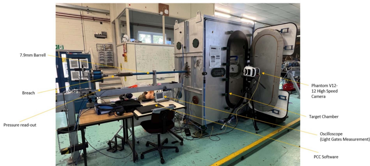
Fig. 5 Gas gun set up.
