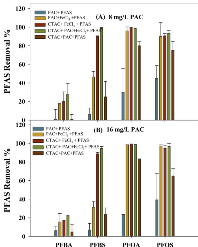
Fig. 4 PFAS removal in Roth Pond water with (A) 8 mg L<sup>-1</sup> and (B) 16 mg L<sup>-1</sup> PAC (blue bar), PAC and coagulant FeCl<sub>3</sub> 100 mg L<sup>-1</sup> (yellow bar), CTAC (1 ppm) spiked with FeCl<sub>3</sub> (red bar), CTAC (1 ppm) spiked with both PAC and FeCl<sub>3</sub> (green bar), and CTAC spiked with PAC (brown bar). Error bars were derived from variants from duplicate experiments.
