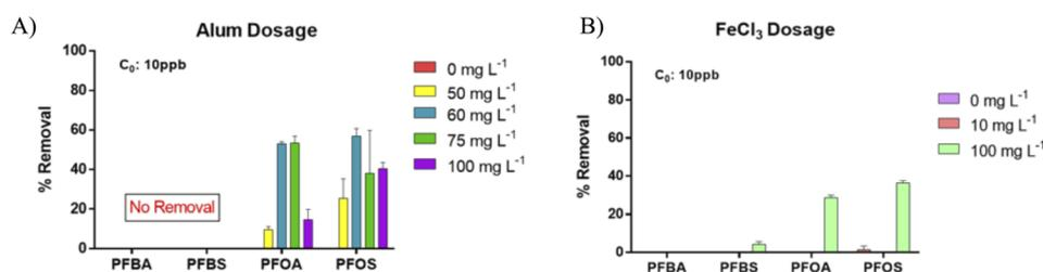
Fig. 1 PFAS removal by conventional and enhanced coagulation. Panel A depicts PFAS removal by various doses of alum coagulant and Panel B depicts PFAS removal by various doses of ferric chloride ( $\text{FeCl}_3$ ) coagulant. Error bars represent mean  $\pm$  SE ( $n = 2$ ).
