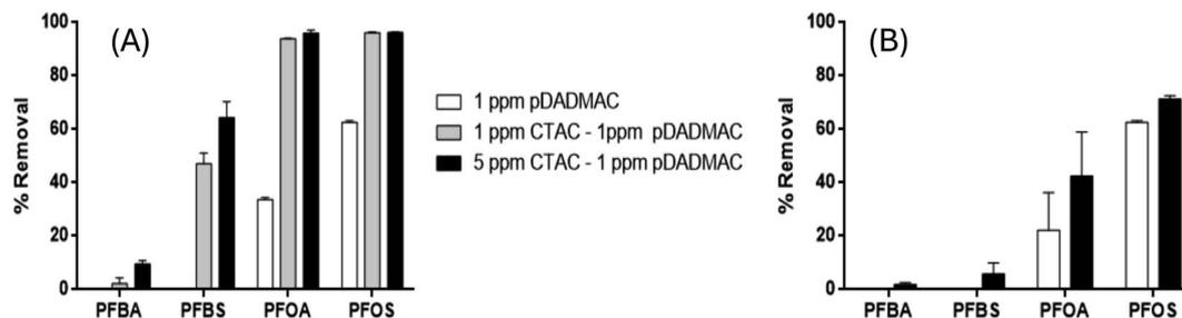
Fig. 3 Additive impact on PFAS removal (in %). Panel A depicts the removal of PFAS by FeCl<sub>3</sub> coagulation in the presence of cationic surfactant CTAC and cationic polymer polyDADMAC. Panel B depicts the removal of PFAS by alum coagulation in the presence of cationic surfactant CTAC and cationic polymer polyDADMAC.
