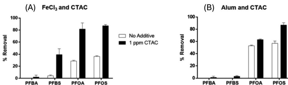
Fig. 2 PFAS removal (in %) by surfactant-enhanced coagulation (A) 100 mg L<sup>-1</sup> of ferric chloride (FeCl<sub>3</sub>) coagulant in the presence and absence of CTAC (1 mg L<sup>-1</sup>); and (B) 60 mg L<sup>-1</sup> of alum coagulant in the presence and absence of CTAC (1 mg L<sup>-1</sup>). Error bars represent mean ± SE (*n* = 2).
