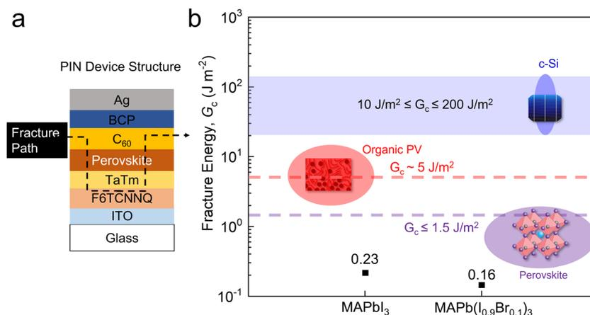
Fig. 2 (a) Device structure and fracture path. (b) The measured average  $G_c$  of the p–i–n samples with MAPbI<sub>3</sub> and MAP(I<sub>0.9</sub>Br<sub>0.1</sub>)<sub>3</sub> in comparison with the  $G_c$  of various PV technologies.
