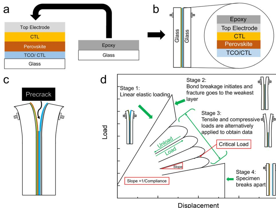
Fig. 1 Schematic illustrations of (a) DCB sample fabrication method, (b) General DCB sample structure (c) Pre-crack (d) Load–displacement response of an ideal fracture energy measurement.
