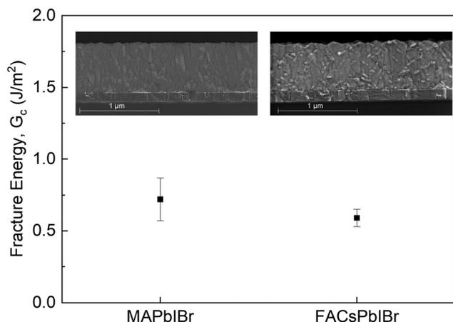
Fig. 4 The measured  $G_c$  of vacuum-evaporated  $\text{MAPb}(\text{I}_{0.9}\text{Br}_{0.1})_3$  and  $\text{FA}_{0.74}\text{Cs}_{0.26}\text{Pb}(\text{I}_{0.86}\text{Br}_{0.14})_3$  perovskites (inset: cross-sectional SEM image of the perovskite layer).
