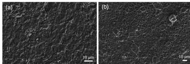
Fig. 5 SEM images of lithium metal coated with a PVDF-HFP : DMF coating (a) before cycling and (b) after 10 cycles in a SPAN pouch cell.
