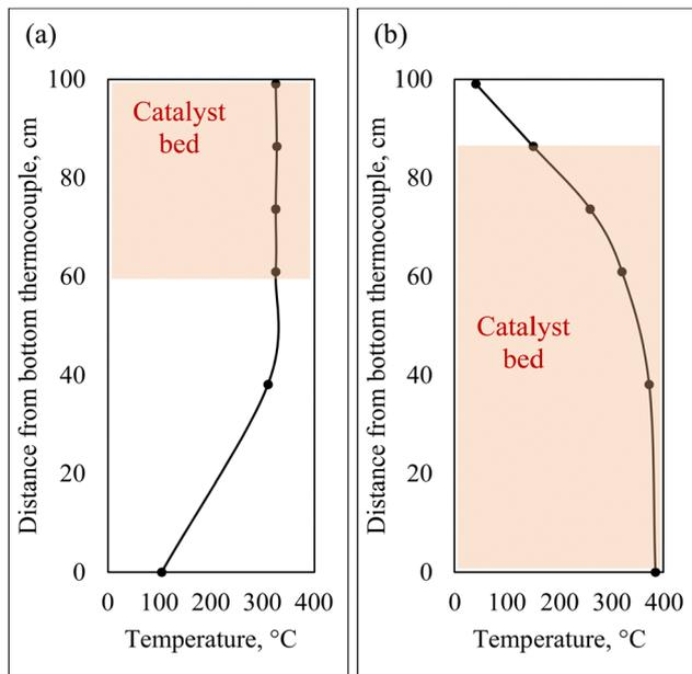
Fig. 2 Hydrotreater reactor temperature profiles and catalyst bed locations: (a) counter-current air flow for co-hydrotreating, (b) co-current air flow for standalone hydrotreating.
