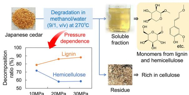
**Effect of process parameters on woody biomass fractionation in a methanol/water mixture in a semi-flow reactor**
