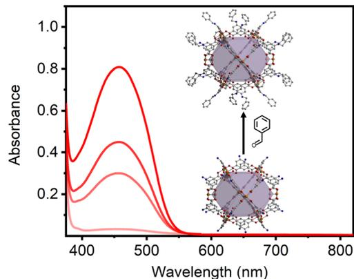
Fig. 3 Reaction of  $\text{Mo}_{24}(\text{5-NH}_2\text{-bdc})_{24}$  with benzaldehyde over the course of four hours with absorbance at 467 nm of 0.03, 0.29, 0.43, 0.79 at 1, 2, 3, and 4, hours, respectively.
