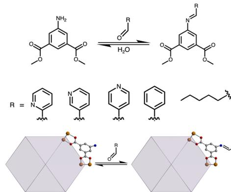
**Fig. 2** Aldehydes utilized in studying the reactivity toward imine functionalization of dimethyl-5- $\text{NH}_2\text{-bdc}$  and a schematic of  $\text{Mo}_{24}(\text{5-NH}_2\text{-bdc})_{24}$  undergoing imine functionalization with corresponding aldehydes. R-CHO, left to right, 2-formylpyridine, 3-formylpyridine, 4-formylpyridine, benzaldehyde, and hexanal.
