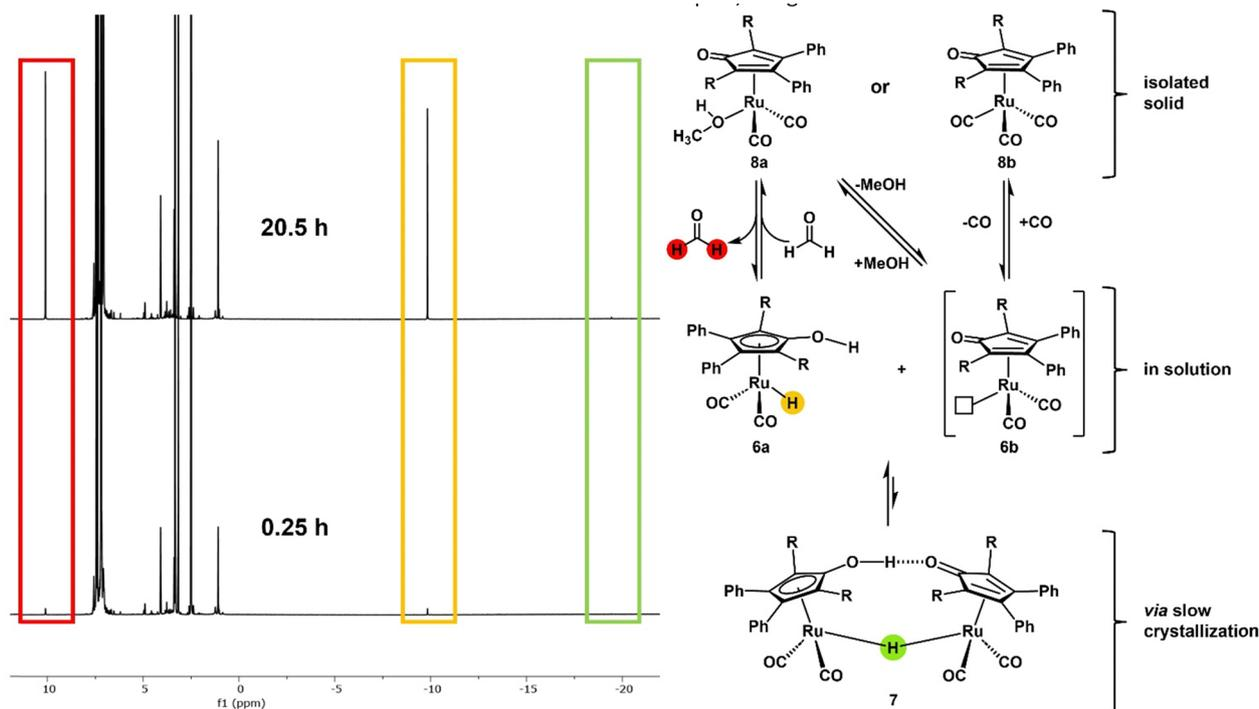
**Fig. 2** Proposed formation of the catalytically active monomeric hydride species **6a** via the dehydrogenation of coordinated and/or residual methanol from the crystals in DMSO- $d_6$  at 25 °C. The  $^1\text{H}$  NMR spectra show the formation of two singlets for formaldehyde (red) and the monomeric hydride **6a** (yellow) over 20.5 h. The spectra show minimal to no formation of the dimeric hydride **7** (green).  $R$  = sodium  $p$ -phenylsulfonate.
