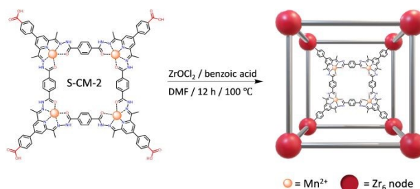
Scheme 2 synthesis of the zirconium-based MOFs using S-CM-2 as building blocks.
